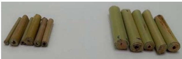
Fig. 2. Small and large diameter samples of bamboos.
