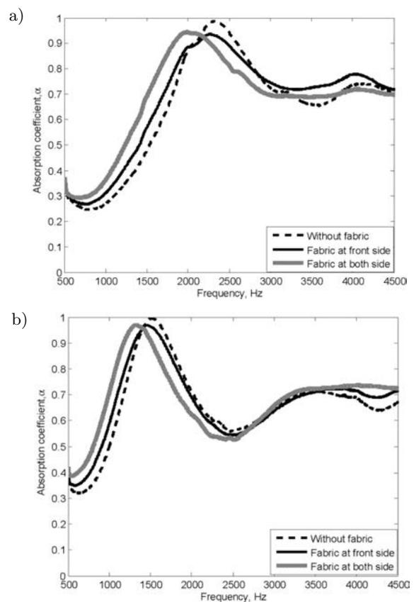
Fig. 13. Absorption coefficient of bamboo in the transverse arrangement with attachment of a fabric for different layer thicknesses: a) 2 cm and b) 3 cm.
