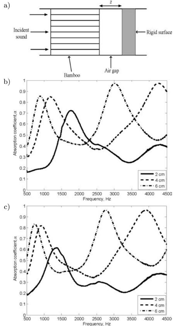
Fig. 7. Absorption coefficient of bamboo in the axial arrangement for different air gaps: a) diagram of the arrangement, b)  $z = 1 \text{ cm}$ , and c)  $z = 2 \text{ cm}$ .
