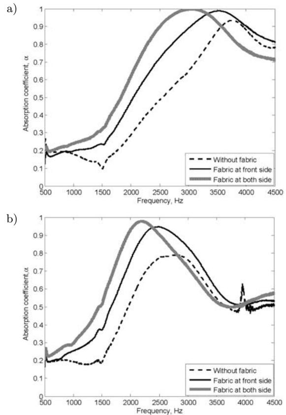
Fig. 10. Absorption coefficient of a large diameter of bamboo with attachment of a fabric for different stem lengths: a) 2 cm and b) 3 cm.
