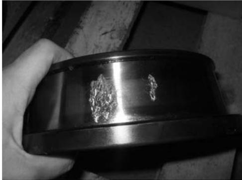
Fig. 16. Spalled inner race of a wind turbine.
