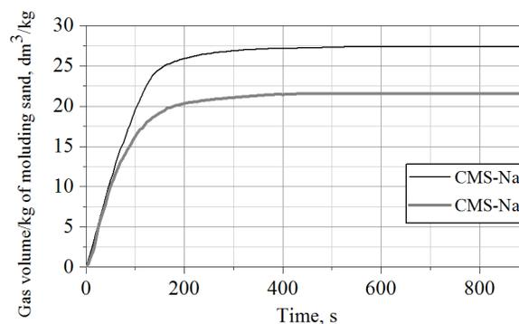
Fig. 1. Emissivity of gases in time from the tested moulding sands after pouring molten cast iron into the mould
