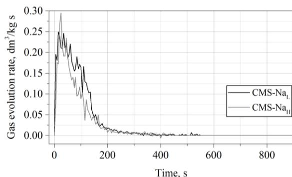
Fig. 2. Gas evolution rate from the tested moulding sands after pouring cast iron into the mould
