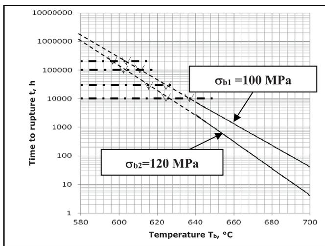
Fig. 1. Results of abridged creep tests of VM12 steel conducted at a temperature higher than the expected operating one and at constant stress level with different values ( $\sigma_{b1} = 100$  MPa;  $\sigma_{b2} = 120$  MPa)
