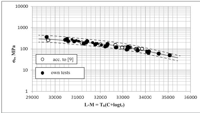
Fig. 2. Parametric average temporary creep strength curve in the form of relationship  $\log \sigma_b = f(L-M)$  for VM12 martensitic steel under investigation. where: L-M is the Larson-Miller parameter;  $L-M = T_b(C + \log t_r)$ ,  $\sigma_b$  – test stress,  $t_r$  – time to rupture,  $T_b$  – test temperature in K,  $C = 37$  – material constant
