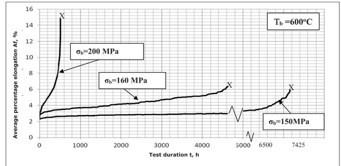
Fig. 4. Comparison of results of creep test with elongation measurement during testing in the form of creep curves  $\epsilon = f(t)$  for different test stress levels  $\sigma_b$  at constant test temperature  $T_b = 600^\circ\text{C}$  for VM12 steel
