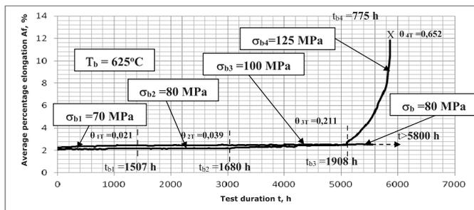
Fig. 7. Comparison of results of creep test with elongation measurement during testing in the form of creep curves  $\varepsilon = f(t)$  for various periodically changed levels of test stress  $\sigma_b$  at constant test temperature  $T_b = 625^\circ\text{C}$  to creep test conducted at constant temperature and stress parameters ( $\sigma_b = 80$  MPa;  $T_b = 625^\circ\text{C}$ ) for VM12 steel
