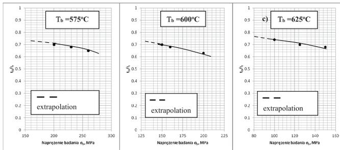
Fig. 6. Share of secondary creep  $t_{II}$  in life time  $t_r$  depending on test creep level at constant test temperature a)  $T_b=575^\circ\text{C}$ , b)  $T_b=600^\circ\text{C}$ , c)  $T_b=625^\circ\text{C}$  for VM12 steel based on creep tests with elongation measurement during testing
