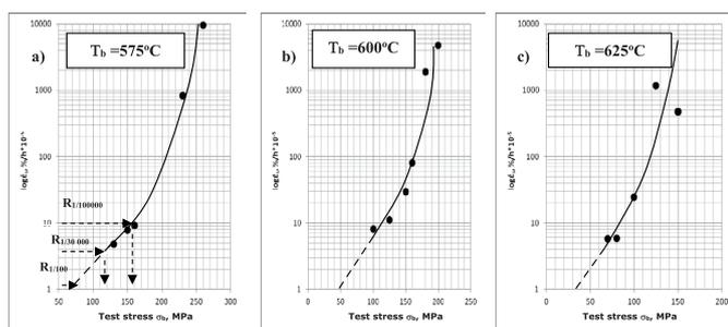
Fig. 9. Steady-state creep rate  $\dot{\epsilon}_s$  as a function of test stress level  $\sigma$  at constant test temperature  $T_b$  of VM12 steel: a) at  $T_b=575^\circ\text{C}$ ; b) at  $T_b=600^\circ\text{C}$ ; c) at  $T_b=625^\circ\text{C}$
