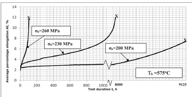
Fig. 3. Comparison of results of creep test with elongation measurement during testing in the form of creep curves  $\epsilon = f(t)$  for different test stress levels  $\sigma_b$  at constant test temperature  $T_b = 575^\circ\text{C}$  for VM12 steel
