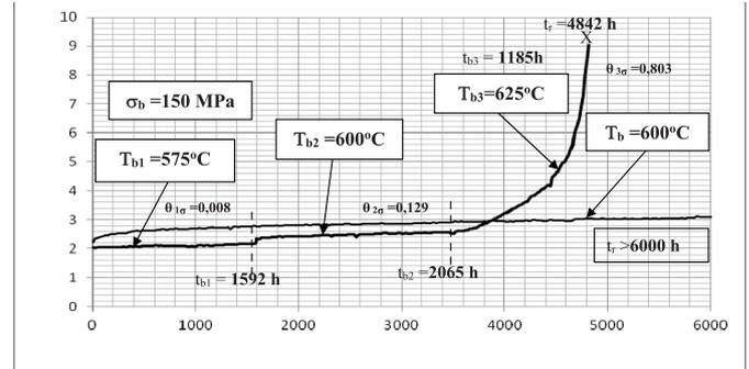
Fig. 8. Comparison of results of creep test with elongation measurement during testing in the form of creep curves  $\varepsilon = f(t)$  for different cyclically changed test temperature levels  $T_b$  at constant test stress level  $\sigma_b = 150$  MPa to creep test conducted at constant temperature and stress parameters ( $\sigma_b = 150$  MPa;  $T_b = 575^\circ\text{C}$ ) for VM12 steel
