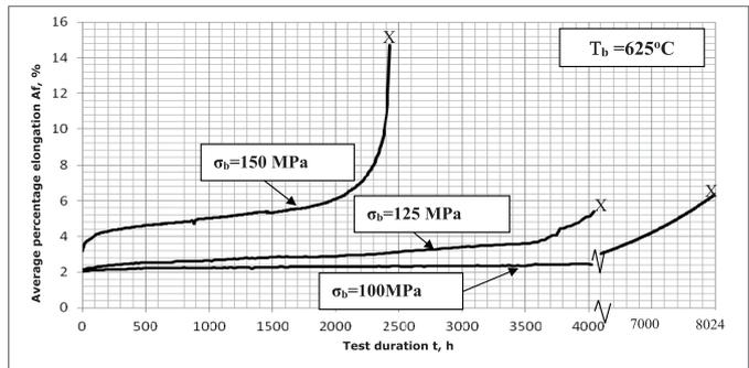
Fig. 5. Comparison of results of creep test with elongation measurement during testing in the form of creep curves  $\epsilon = f(t)$  for different test stress levels  $\sigma_b$  at constant test temperature  $T_b = 625^\circ\text{C}$  for VM12 steel
