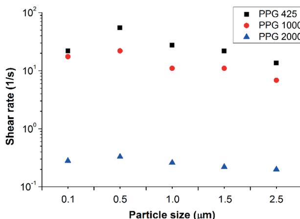
Fig. 3. Shear rate at maximum of shear thickening depending on particle size of ceramic powder
