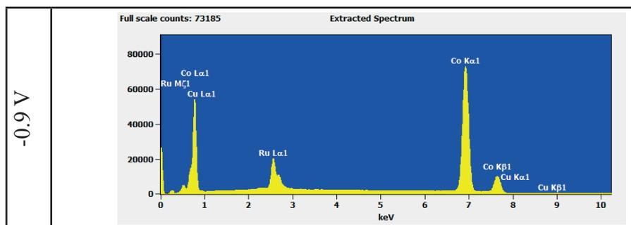
Fig. 6. Qualitative scanning analysis of elements in alloys obtained from electrolyte containing 10 mM  $\text{RuCl}_3$ , 100 mM  $\text{CoCl}_2$  at different deposition potentials.
