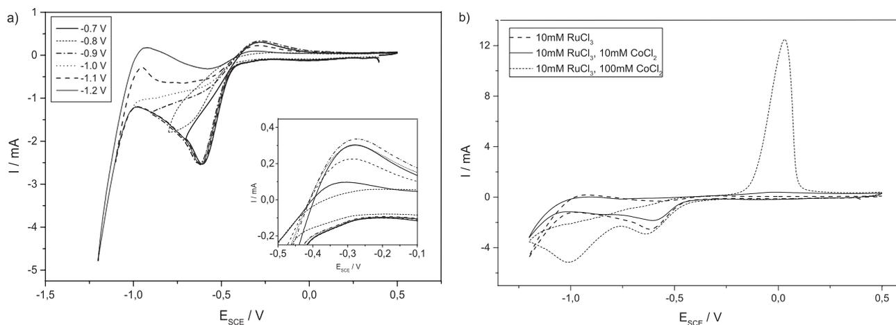
Fig. 1. Voltammetric curve made for solutions: a) 10 mM  $\text{RuCl}_3$ , 1M  $[\text{Cl}^-]$ , pH = 1 at different scanning range, b) 10 mM  $\text{RuCl}_3$ , 10 mM  $\text{CoCl}_2$  and 10 mM  $\text{RuCl}_3$ , 100 mM  $\text{CoCl}_2$ , 1M  $[\text{Cl}^-]$ , pH = 1
