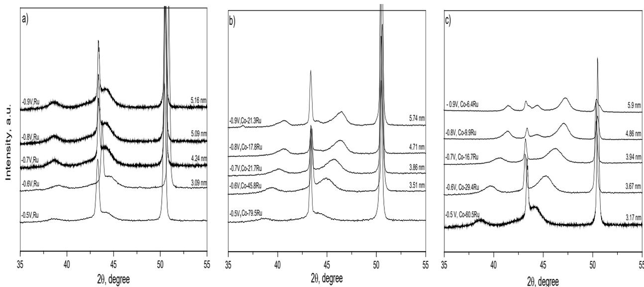
Fig. 3. X-ray diffraction patterns of coatings obtained from electrolytes composed of a) 10 mM  $RuCl_3$  b) 10 mM  $RuCl_3$  + 10 mM  $CoCl_2$  c) 10 mM  $RuCl_3$  + 100 mM  $CoCl_2$  and deposition potential ranges from -0.5 to -0.9 V vs SCE. The diagram also includes composition of a Co-Ru alloy and sizes of crystallites
