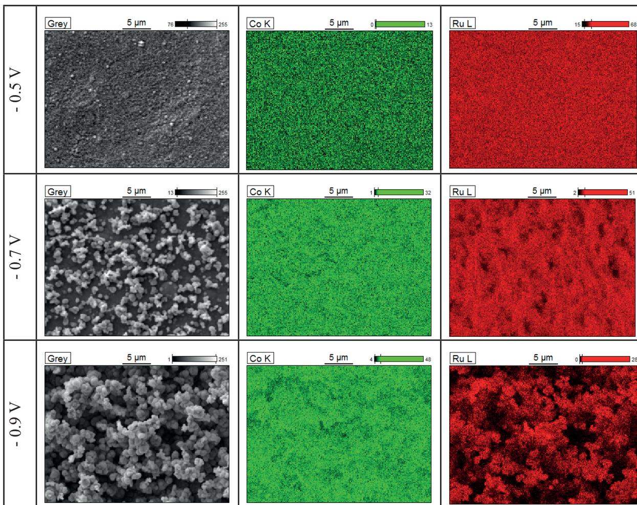
Fig. 5 SEM photograph presents a structure and elemental distribution of the obtained coatings quantified in 4000X, obtained from electrolyte containing 10 mM RuCl<sub>3</sub>, 100 mM CoCl<sub>2</sub> at different deposition potentials
