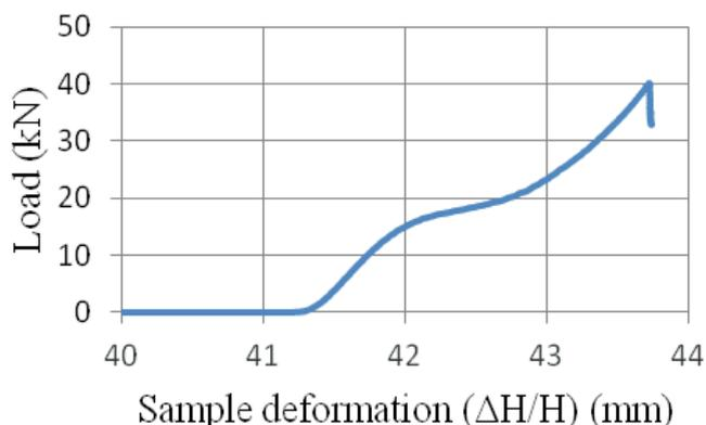
Fig. 13. Compression curve for temperature of 60°C
