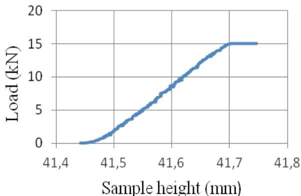
Fig. 4. Change of sample height under the influence of applied load of 15 kN at temperature of 40°C
