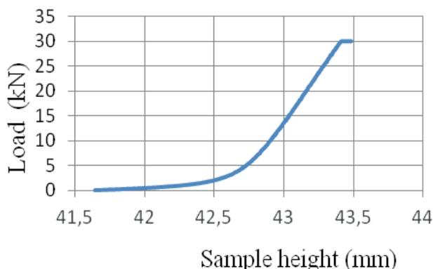
Fig. 10. Change of sample height under the influence of applied load of 30 kN at temperature of 80°C
