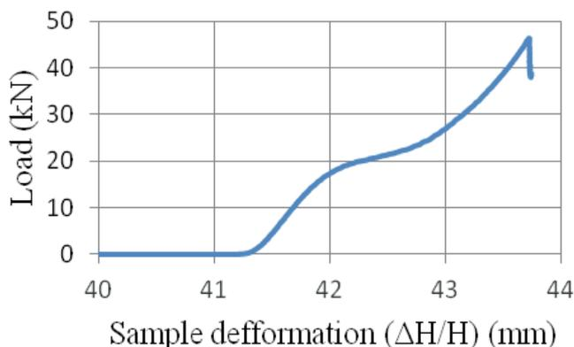
Fig. 12. Compression curve for temperature of 40°C
