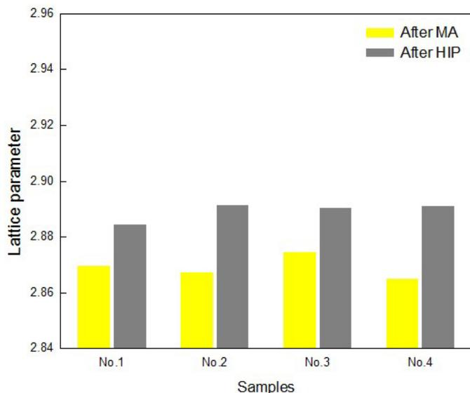
Fig. 2. Lattice parameter of Fe after MA and HIPing for specimen No.1~4 : (a)~(d)
