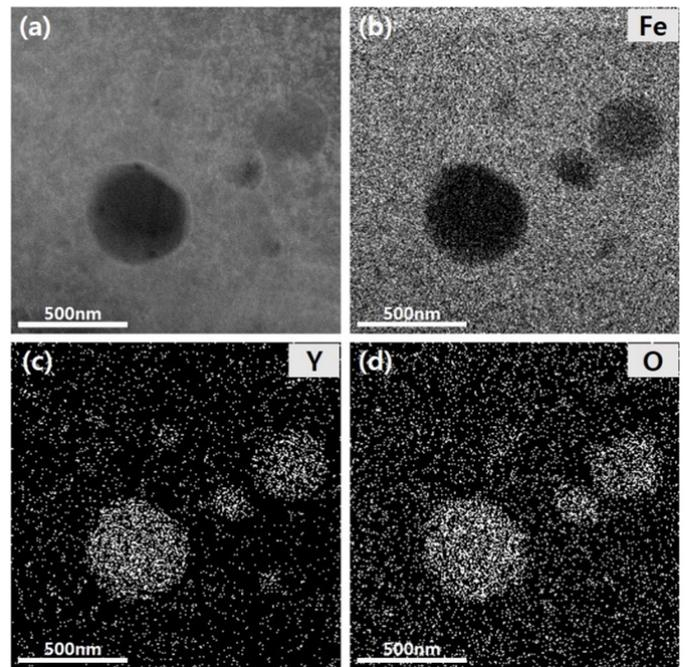
Fig. 6. TEM/EDS results of the Fe-2Y<sub>2</sub>O<sub>3</sub> alloy (specimen No. 3) after HIPing
