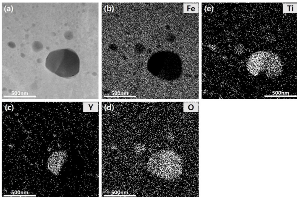
Fig. 7. TEM/EDS results of the Fe-2Y<sub>2</sub>O<sub>3</sub>-0.5Ti alloy (specimen No.4) after HIPing
