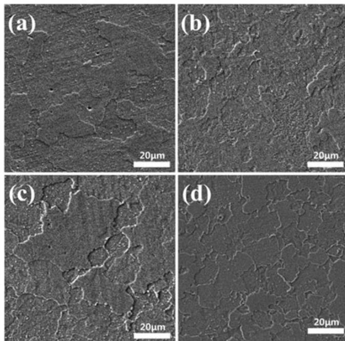
Fig. 4. SEM micrographs after HIPing for specimen No.1~4 : (a)~(d)
