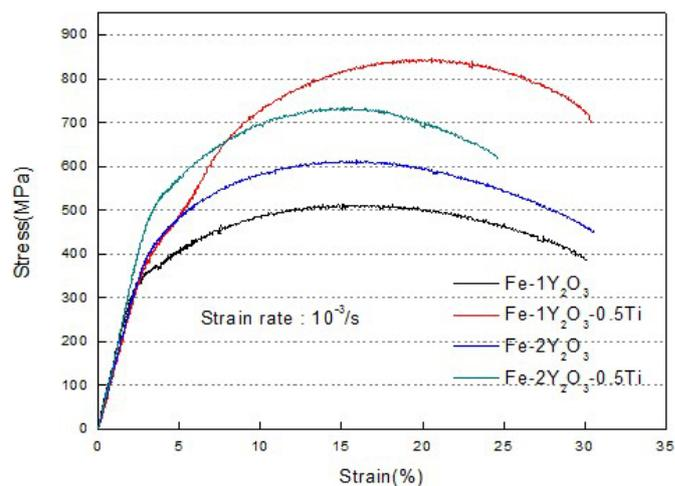
Fig. 5. Tensile curves for alloys after HIPing
