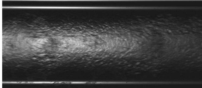
Figure 11: Experimentally obtained dryout adiabatic flow of R134a for  $G = 400 \text{ kg/m}^2\text{s}$  with  $\dot{q} = 39 \text{ kW/m}^2$ , point D on flow pattern map.
