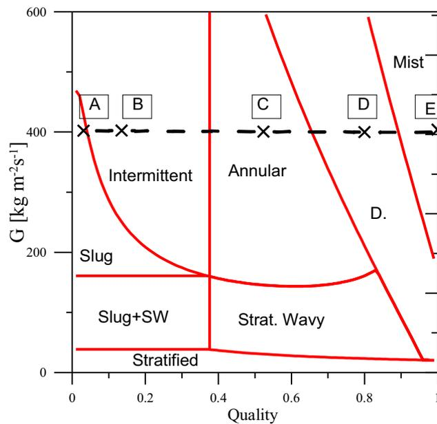
Figure 7: Flow pattern map evaluated for R134a at  $T_{sat} = 19.4 \text{ }^\circ\text{C}$  in a 5 mm internal diameter tube for  $\dot{q} = 35 \text{ kW/m}^2$  using  $G = 400 \text{ kg/m}^2\text{s}$  to calculate the void fractions.
