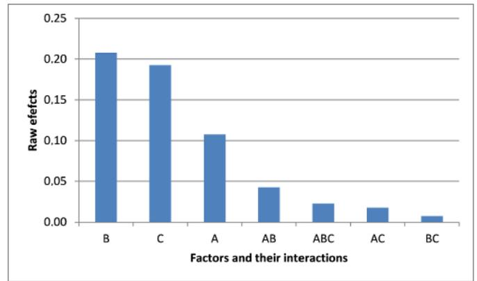
Fig. 8. Pareto chart for the raw effects analysis of the friction coefficient. Codes: A – a laser treatment (yes vs. no), B – a load (5 N vs. 15 N), C – a lubrication (nothing vs. oil); multi-characters – respective interactions
