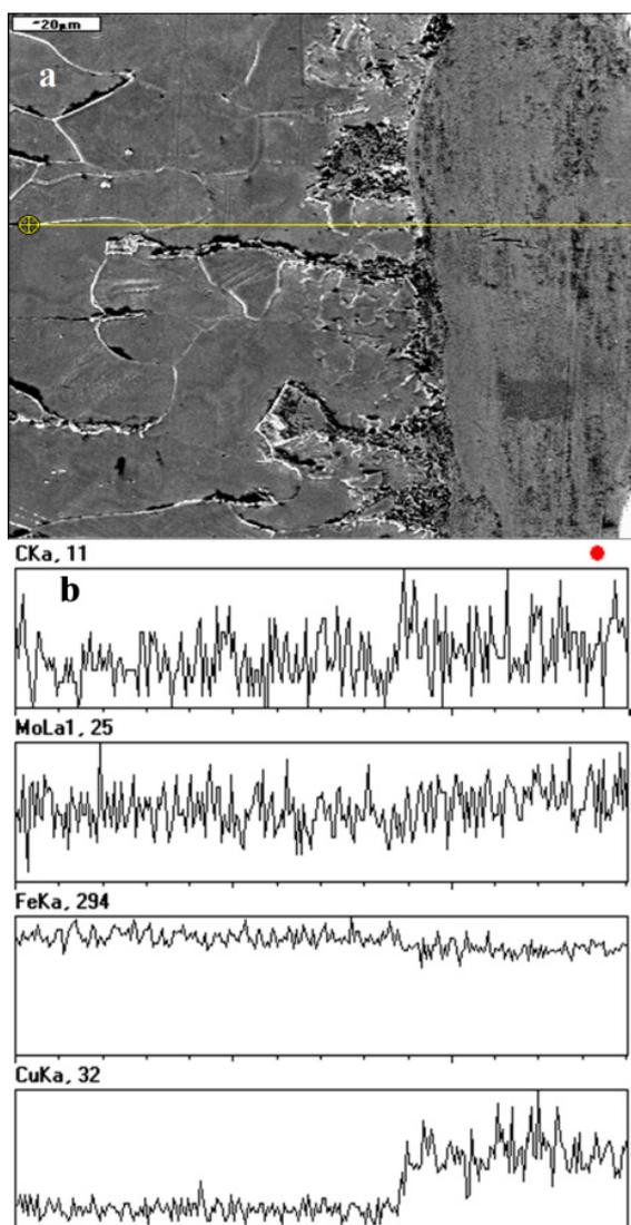
Fig. 2. Microstructure (a) and linear distribution of elements (b) in the Cu-Mo coating after laser treatment (scale marker: 20  $\mu\text{m}$ )
