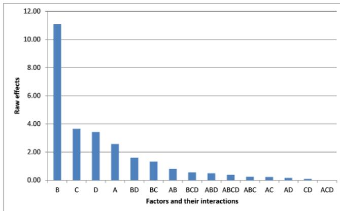
Fig. 7. Pareto chart for the raw effects analysis of the mass loss. Codes: A – a laser treatment (yes vs. no), B – a load (5 N vs. 15 N), C – a lubrication (nothing vs. oil), D – a geometric form (pin vs. disc); multi-characters – respective interactions
