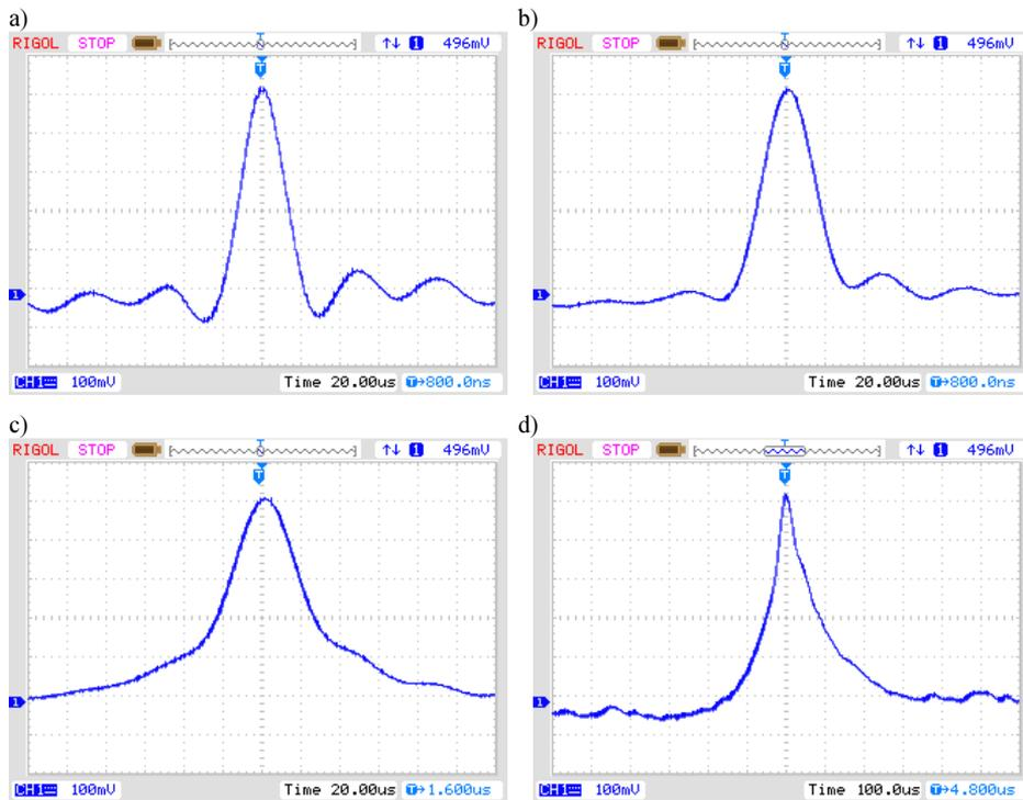
Fig. 4. The behaviour of functions of CAV: the low-pass white noise:  $N(0 \text{ V}, 0.3 \text{ V})$ ,  $B = 25 \text{ kHz}$  and after the noise passed the first-order inertial system with various time constants  $T_c$ : (a)  $T_c = 10 \mu\text{s}$  (b);  $T_c = 30 \mu\text{s}$  (c);  $T_c = 100 \mu\text{s}$  (d).
