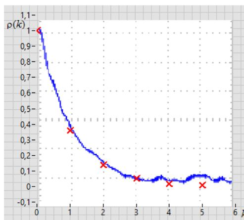
Fig. 5. The experimental behaviour of normalized autocorrelation function  $\rho_x(k\Delta t)$  of the low-pass white noise  $N(0 \text{ V}, 0.3 \text{ V})$ ,  $B = 25 \text{ kHz}$  after it passed the first-order inertial system with a time constant  $T_c = 100 \mu\text{s}$  (continuous line) and the calculated autocorrelation values (points x).
