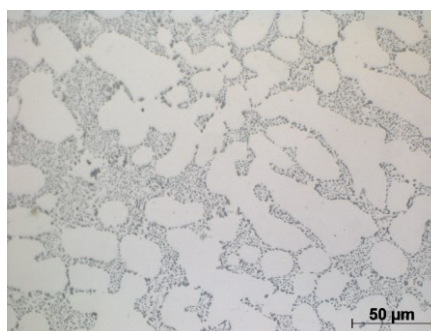
Fig. 4. The as cast microstructure of AlSi10Mg(Cu) alloys
