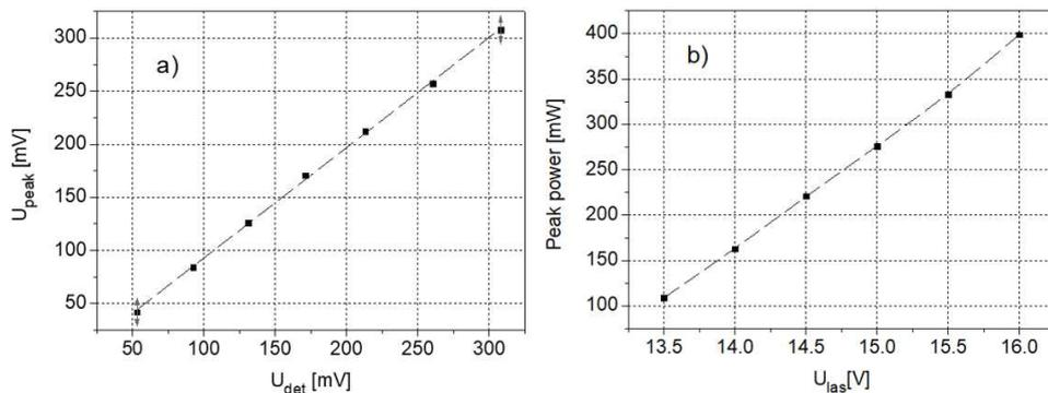
Fig. 9. Processing characteristics of the monitoring unit (a) and control characteristics of QCL laser (b).
