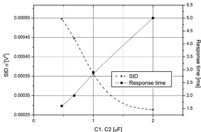
Fig. 5. The influence of the  $C_1$ ,  $C_2$  capacities on standard deviation of the output voltage and the response time of the peak monitoring unit.
