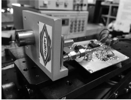
Fig. 6. A photo of the detection module with the developed monitoring unit.
