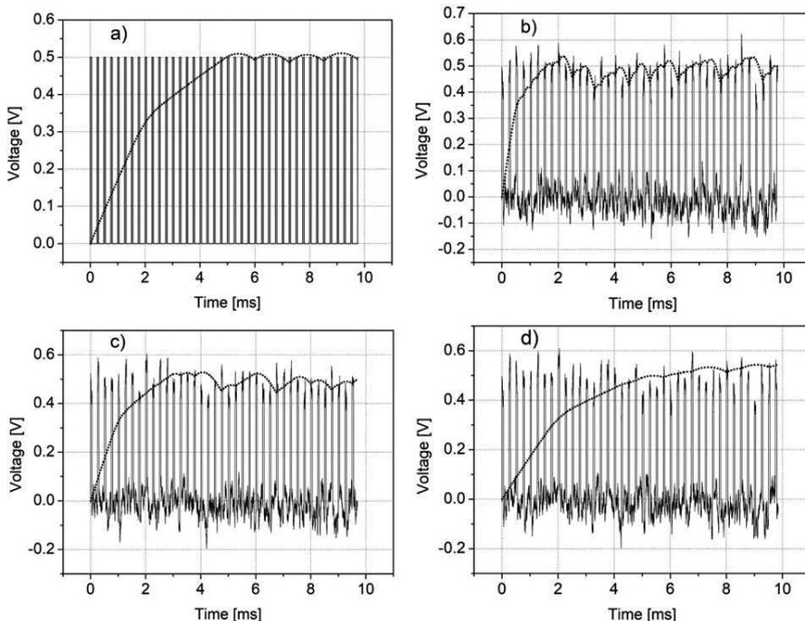
Fig. 4. Response signals of the monitoring unit for: a) a noiseless reference signal and  $C_2 = 2 \mu\text{F}$ ; b) a noisy signal for  $C_2 = 470 \text{ nF}$ ; c) a noisy signal for  $C_2 = 1 \mu\text{F}$ ; d) a noisy signal for  $C_2 = 2 \mu\text{F}$ .
