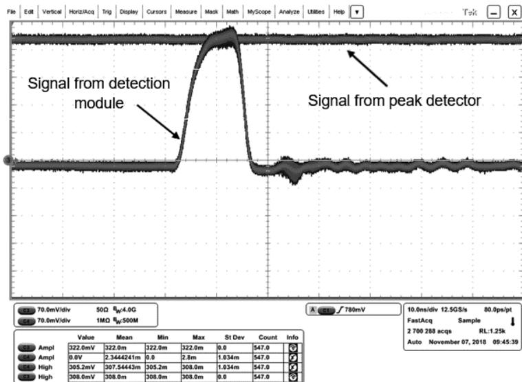
Fig. 8. A pulse shape registered with the detection module and an output signal from the monitoring unit.
