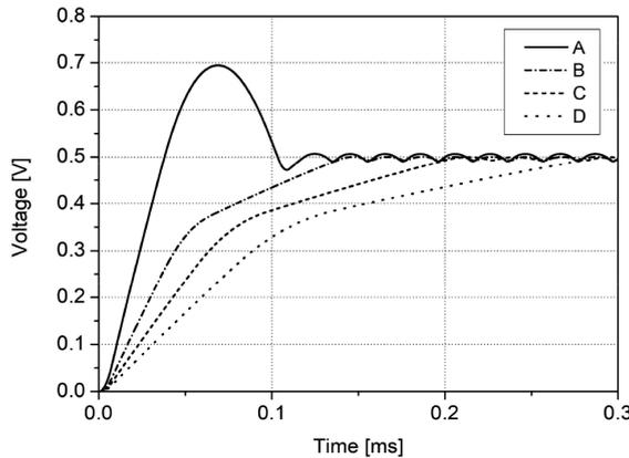
Fig. 3. Simulation responses of the peak detector for  $C_2$  capacities of 220 nF (B), 330 nF (C), 470 nF (D). "A" curve was obtained with  $C_2 = 220$  nF and a low value of  $R_6 = 1$  k.
