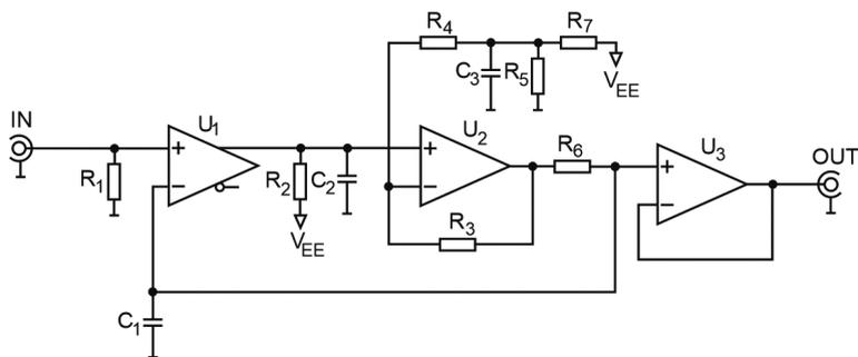
Fig. 2. A peak detector circuit for monitoring the pulse power.
