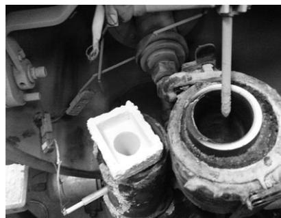
Fig. 3. Chamber of VSG-02 induction furnace
