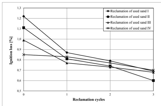
Fig. 3. Ignition losses of the tested mixtures of spent sands and their reclaims
