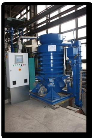
Fig. 1. The prototype vibratory reclaimer REGMAS
