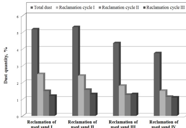
Fig. 2. Results of dusts amounts generated in the spent sands regeneration process, SPENT SAND I- SPENT SAND IV in the REGMAS reclaimer
