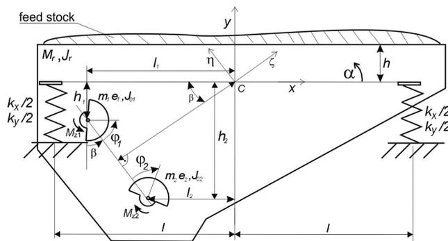
Fig. 1. Schematic presentation of the typical vibratory machine with two vibrators
