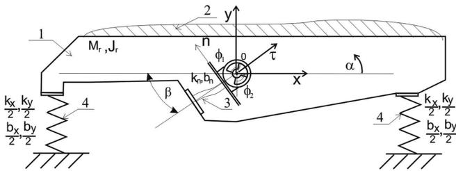
Fig. 3. Conveyor with vibrators situated in the centre of gravity of the main mass
