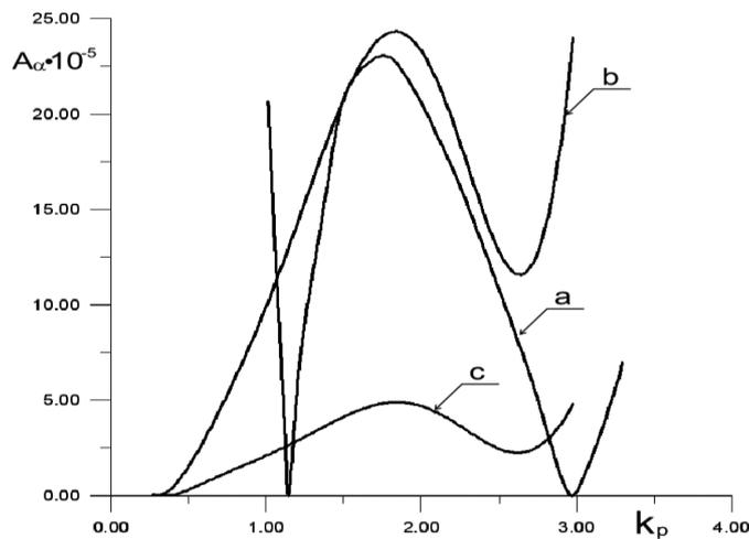
Fig. 5. Dependence of the amplitude of the body oscillations  $A_\alpha$  on the coefficient of throw  $k_p$ , for loose feed of a mass 60 kg: a) Theoretical curve, b) Diagram obtained by the numerical simulation of the classical conveyor, c) Diagram obtained by the numerical simulation of the new conveyor
