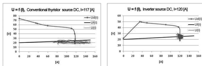
Fig. 2. The example of static real characteristics of the welding power source  $U_d(I)$  Conventional arc characteristic  $U_f(I) = 20 + 0,04I$ , real arc operation  $U(I)$ , Welding power source: conventional thyristor rectifier and inverter equipment. Electrode: E 380 R 11,  $\phi 3,2 \times 350$  mm
