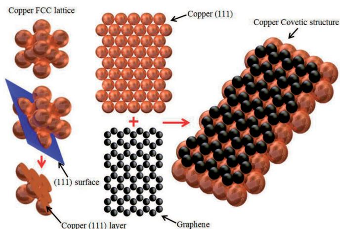
Fig. 1. Idea of copper Covetic material nanoscale structure
