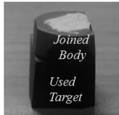
Fig. 4. ITO green body joined with used target by sintering at 1300°C for 2 h under 0.296 MPa
