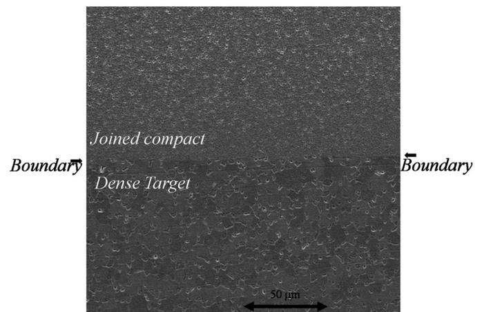
Fig. 5. Boundary between ITO green body and dense target joined by sintering at 1300°C for 2 h under 0.296 MPa
