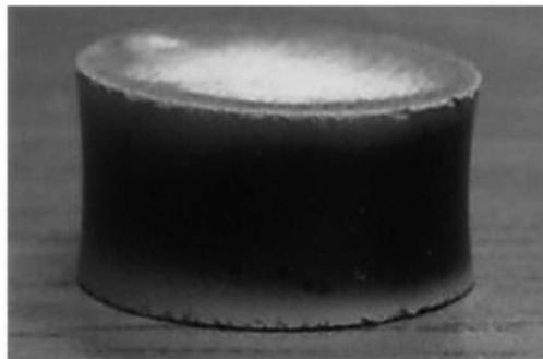
Fig. 7. ITO green body sintered at 1300°C for 2 h under the 0.296 MPa
