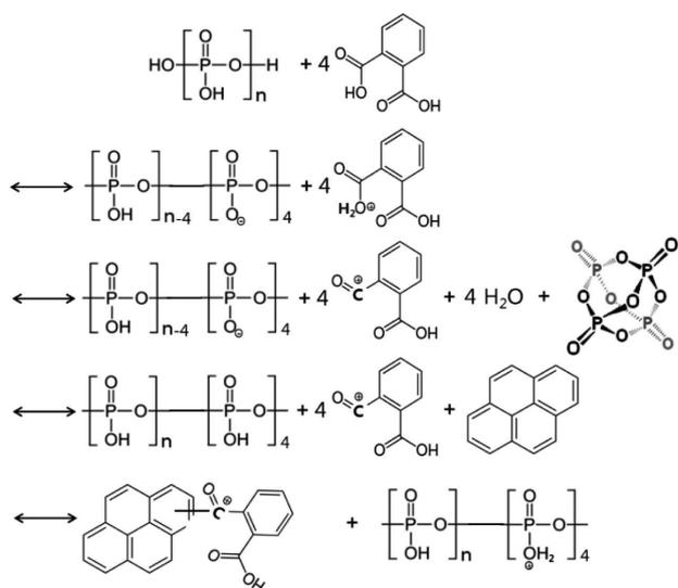
Fig. 3. Functionalization mechanism of graphite using phthalic acid
