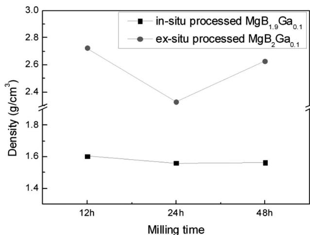
Fig. 7. Effect of milling time on the sintered density of samples. (No.1~6)
