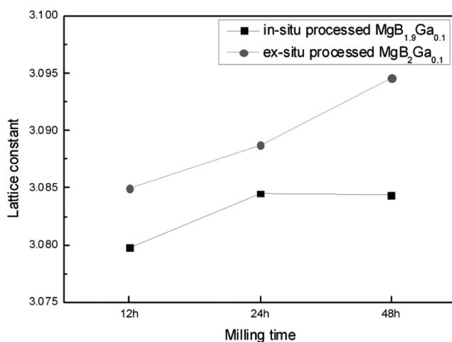
Fig. 8. Effect of milling time on the lattice parameter  $a$  of  $\text{MgB}_2$  phase
