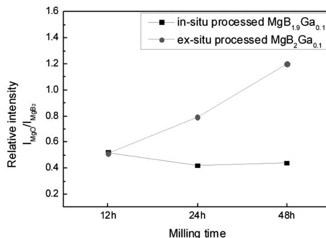
Fig. 3. Relative XRD peak intensity of MgO(200)/MgB<sub>2</sub>(101)
