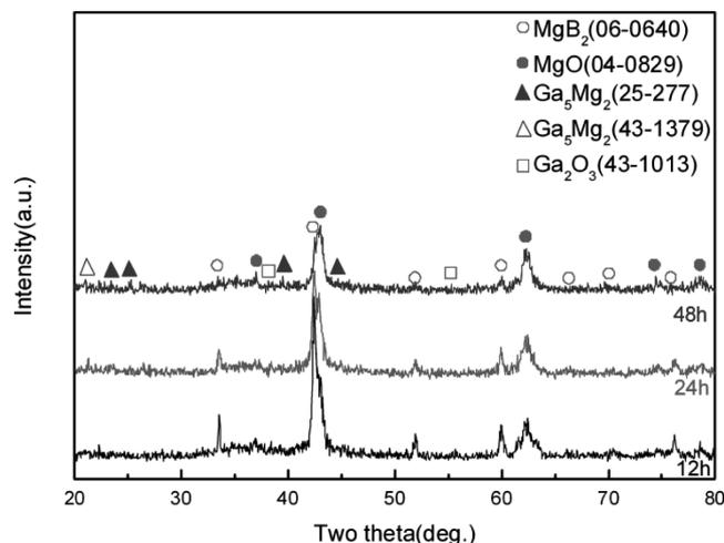
Fig. 2. XRD patterns of ex-situ processed MgB<sub>2</sub>Ga<sub>0.1</sub>. (No.4~6) (Time: ball-milling duration)
