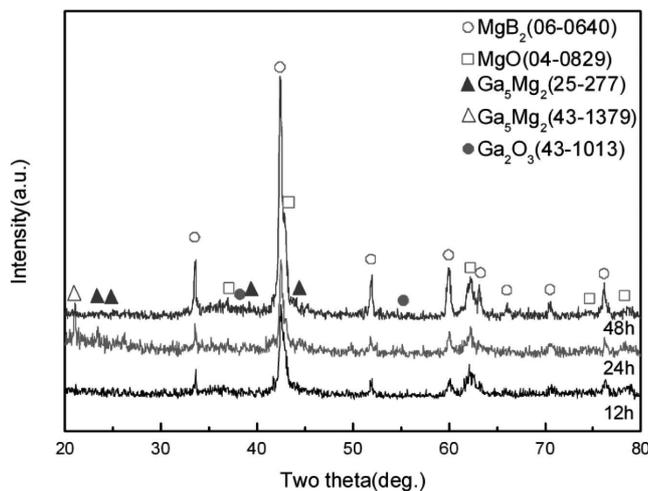
Fig. 1. XRD patterns of in-situ processed MgB<sub>1.9</sub>Ga<sub>0.1</sub>. (No.1~3) (Time: ball-milling duration)
