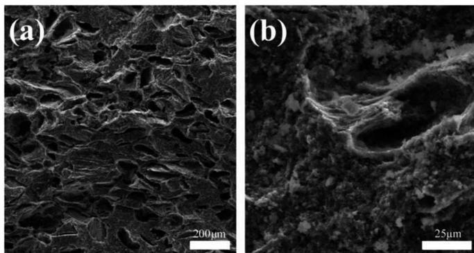
Fig. 4. Fractured surface images of sintered MgB<sub>2</sub>. (b): higher magnification image)
