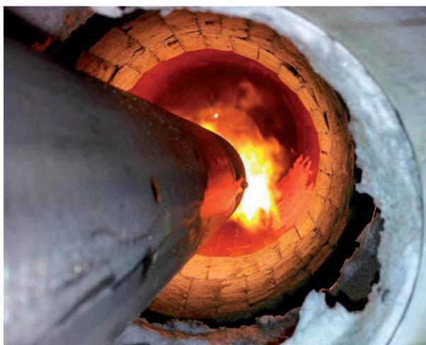
Fig. 2. Rotary kiln equipped with oxygen burner
