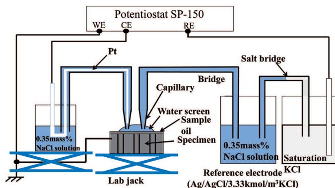
Fig. 1. Schematic diagram of apparatus for the polarization curve measured
