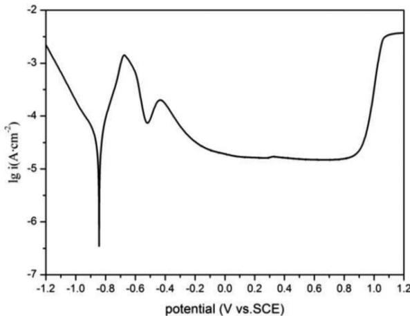
Fig. 2. The potentiodynamic polarization curve of X80 in 0.5M Na<sub>2</sub>CO<sub>3</sub>-1M NaHCO<sub>3</sub> solution
