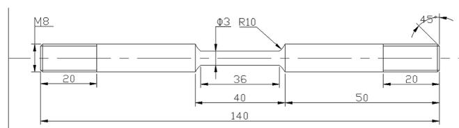
Fig. 1. Schematic diagram of specimens for the samples of SSRT tests
