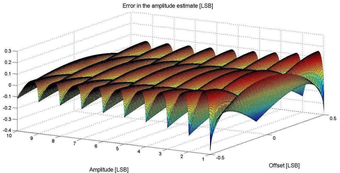
Fig. 2. The estimation error of the sine wave amplitude after the quantization as a function of the amplitude and the offset.
