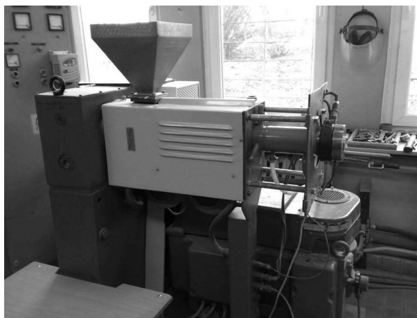
Fig. 1. Modified single screw extrusion-cooker TS-45, equipped with electric heaters and air-water cooling system of the barrel
