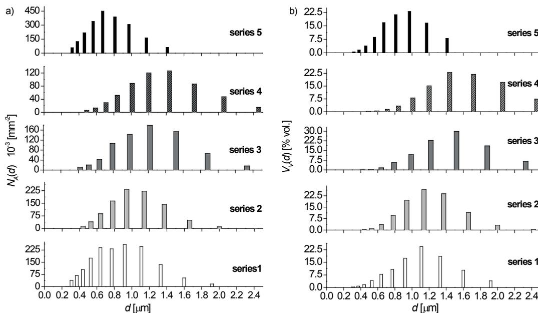
Fig. 2. The grain size distribution a) the dependence of the  $N_A$  grain number of a given size on the unit area on the  $d$  grain size (the statistical distribution), b) the dependence of the  $V_V$  grain volume of a given size on the  $d$  grain size (the geometrical distribution)
