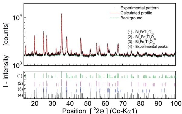
Fig. 3. X-ray diffraction matching parameters for  $\text{Bi}_6\text{Fe}_2\text{Ti}_3\text{O}_{18}$  ceramics fabricated via solid state reaction route and pressureless sintering at  $T=1080^\circ\text{C}$ ; (bottom plot – peak positions of the experimental pattern and the main reference phases)
