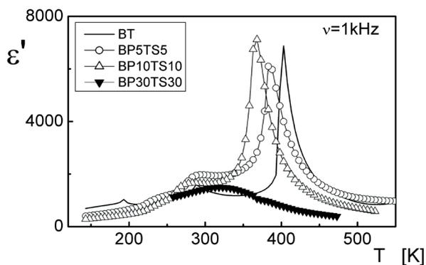
Fig. 2 Temperature dependence of the real part of dielectric permittivity  $\epsilon'$  for BT, BPTS5, BPTS10 and BPTS30 samples
