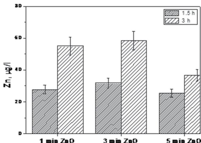
Fig. 2. The release of zinc from modified titanium samples after 1.5 h and 3 h incubation in distilled water.
