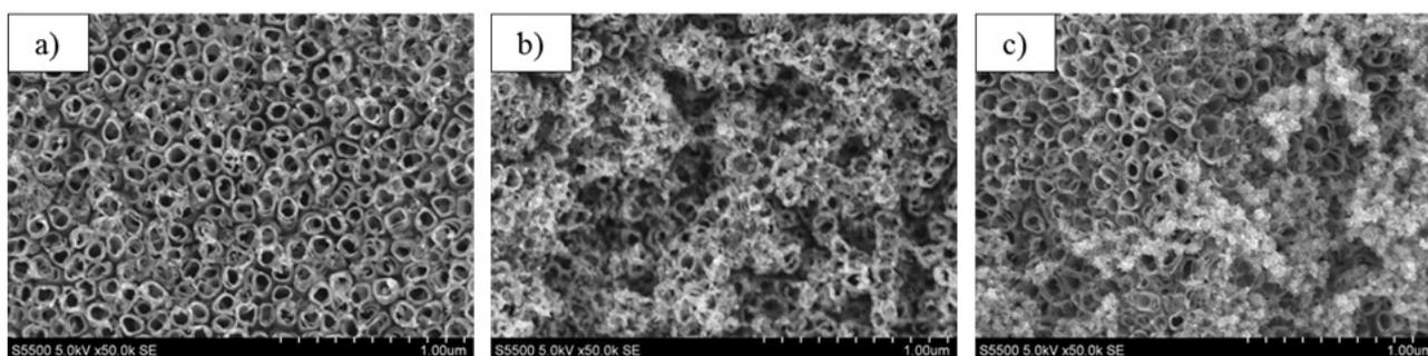
Fig. 1. SEM images of ZnO nanoparticles electrodeposited on TiO<sub>2</sub> nanotubes-modified titanium surfaces for 1 min. (a), 3 min. (b) or 5 min. (c).
