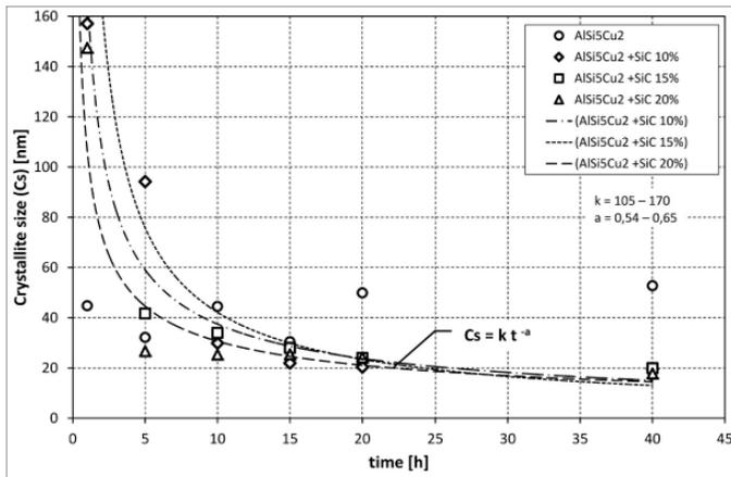
Fig. 3. Crystallite size of powder mixture after different time of mechanical alloying
