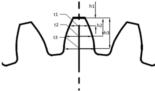
Fig. 10. Places of the thickness measurement of teeth
