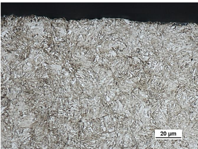
Fig. 3. Microstructure of the surface layer of AMS6265 steel after low pressure carburizing with oil hardening
