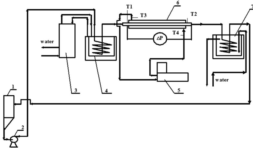
Figure 1: Experimental set-up. 1 – nanofluid container, 2 – pump, 3 – chiller, 4 – secondary cooler, 5 – thermostat, 6 – shell-tube heat exchanger, 7 – primary cooler,  $T_1, T_2, T_3, T_4$  – K-type thermocouples,  $\Delta P$  – pressure transducer.
