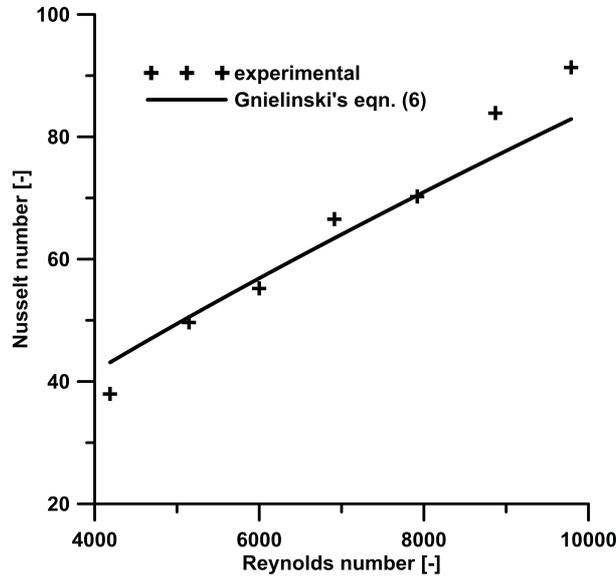
Figure 2: Comparison of experimental and calculated Nusselt number.
