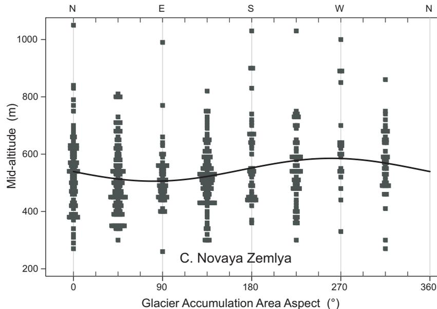
Fig. 8. Variation of mid-altitude with aspect for all glaciers in central Novaya Zemlya, 72.8° to 74.65° N. Glaciers are lowest facing  $081^\circ \pm 22^\circ$ :  $\text{Mid-altitude} = 546 - 6 \cos(\text{aspect}) - 39 \sin(\text{aspect})$ ;  $R^2 = 4\%$ ,  $\text{rmse} = 124 \text{ m}$ ,  $p = 0.0001$ ,  $n = 486$ .
