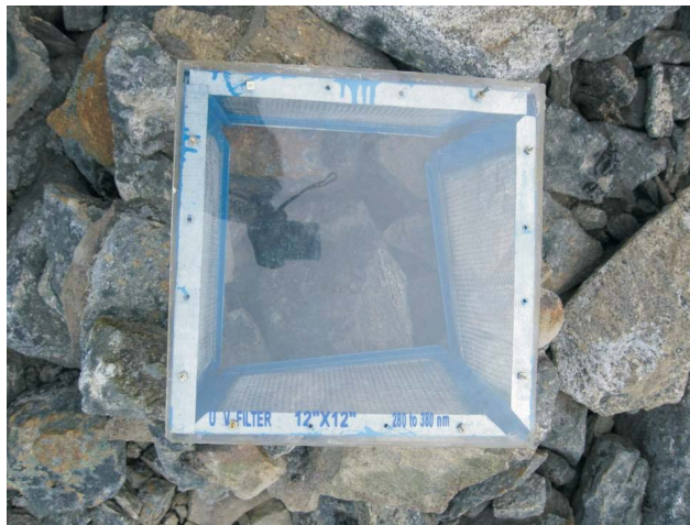
Fig. 1. UV filter frame used for controlled experimental set up.
