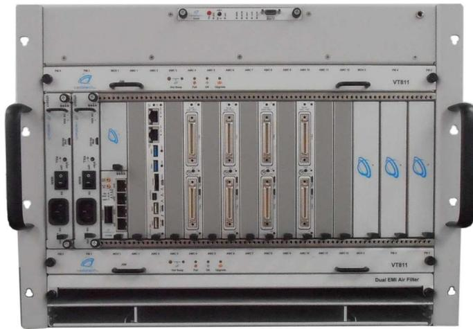
Fig. 3. Example MTCA system for MAST Tokamak [6]
