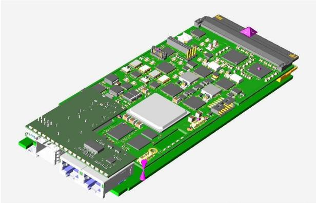
Fig. 8. view of WR-MCH module (PCle hub module not visible)
