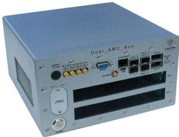
Fig. 4. Miniature MTCA case for two AMC modules [6]
