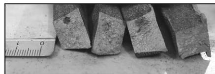
Fig. 4. Result of Althoff-Radtke test for sample modified 0.25% Fe-Ti; respectively, from the left arm length 50, 150, 250, 350 mm
