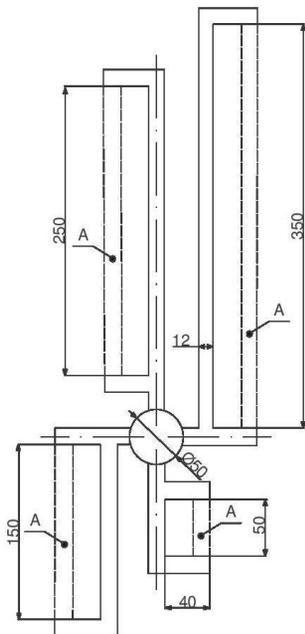
Fig. 1. Standardized form for Althoff-Radtke test [9]
