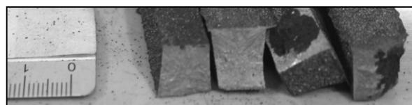
Fig. 5. Result of Althoff-Radtke test for sample modified 0.5% Fe-Ti; respectively, from the left arm length 10, 150, 250, 350 mm
