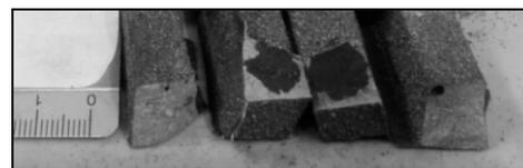
Fig. 6. Result of Althoff-Radtke test for sample modified 0.75% Fe-Ti; respectively, from the left arm length 50, 150, 250, 350 mm
