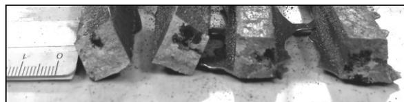
Fig. 3. Result of Althoff-Radtke test for reference sample; respectively, from the left arm length 50, 150, 250, 350 mm
