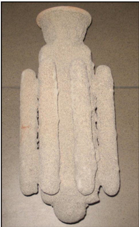
Fig. 1. Ceramic mould for strength tests casts
