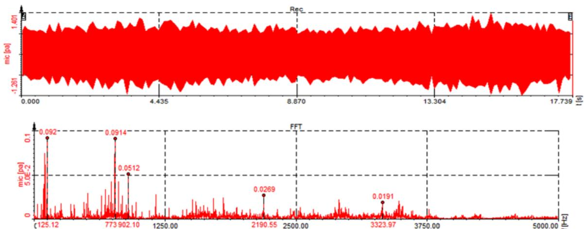
Fig. 2. AE signal of Good bearing
