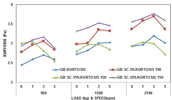
Fig. 4c. KURTOSIS graph for 150 μm particle size
