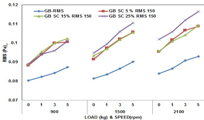
Fig. 3c. RMS graph for 150 μm particle size
