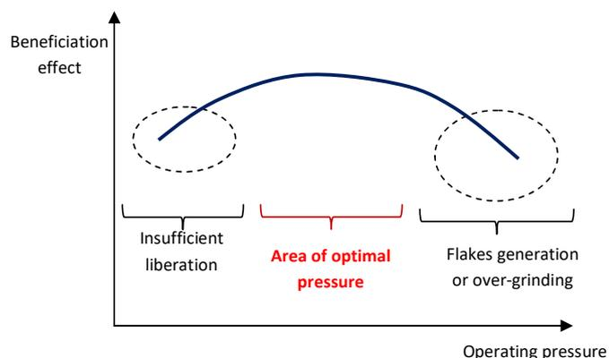
Fig. 1. Parabolic relationship between the operating pressure and beneficiation effect
