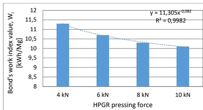
Fig. 9. Bond's work index value for HPGR products crushed at various operating pressure
