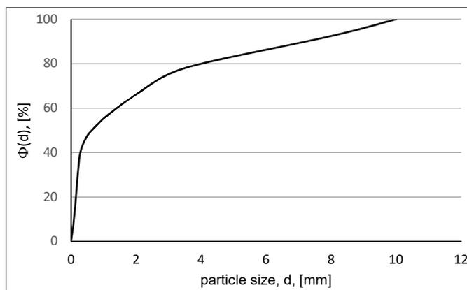
Fig. 2. Particle size composition of HPGR feed material
