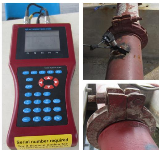
Fig. 3. MultiSystem 5060 portable tester
