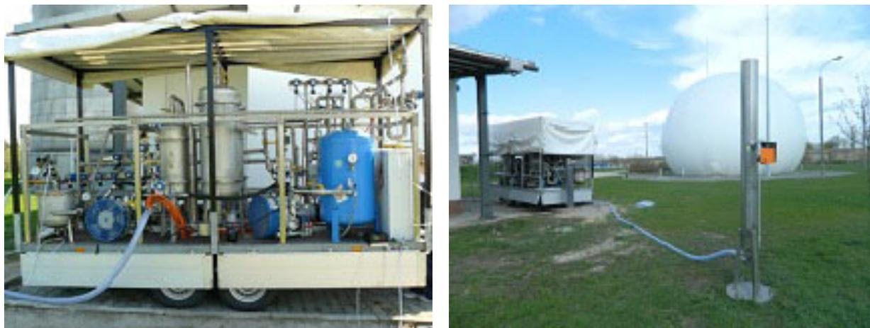
Fig. 4. Photo of the setup at field experiment at biogas installation at municipal wastewater treatment plant. General view of MMI installed on mobile deck (left), fabric raw biogas tank, MIM and biogas flare (right). The municipal wastewater sludge biogas plant testing case
