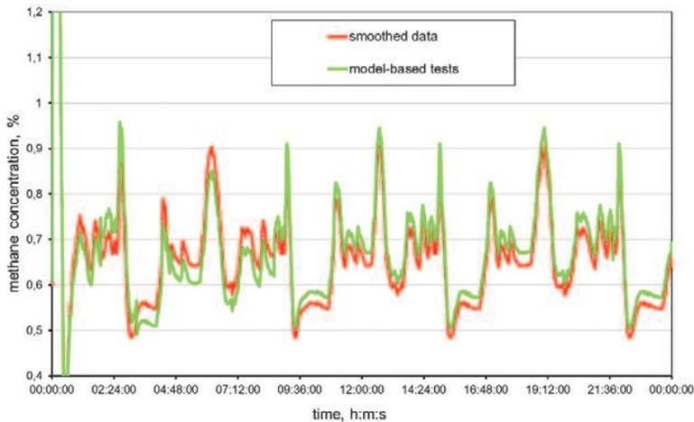
Figure 7: Comparison of methane concentration values obtained from measurements (smoothed data) and model-based tests in the MWR-3 measurement point
