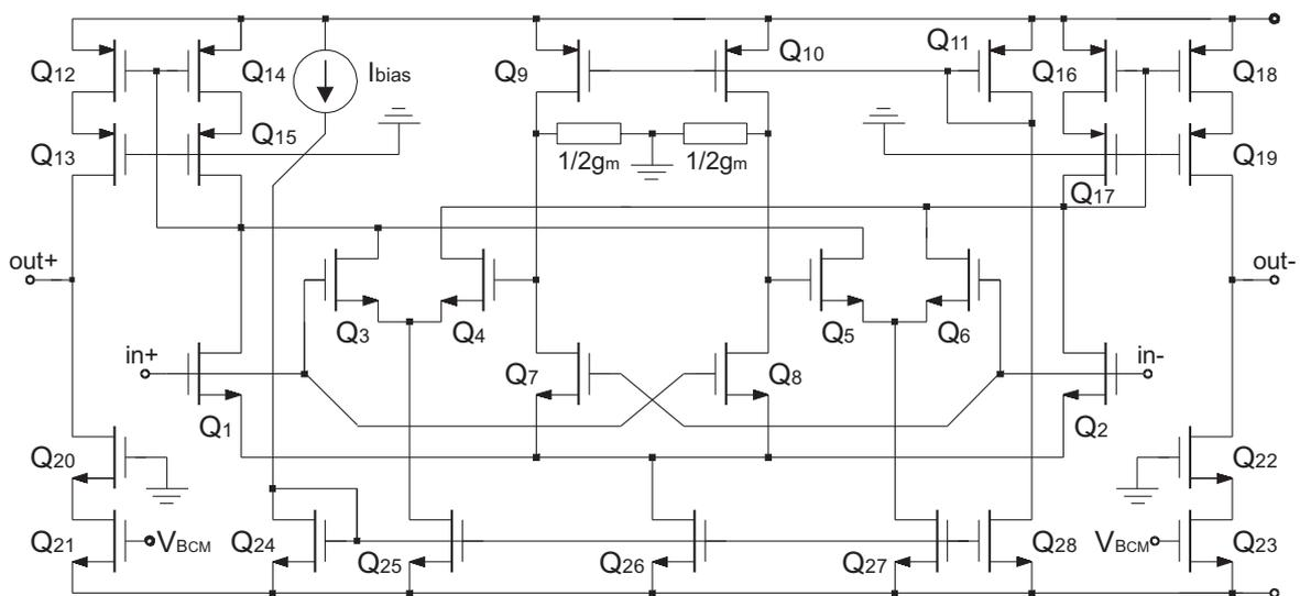
Fig. 9. Complete diagram of the linearized CMOS OTA
