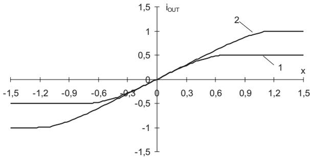
Fig. 5. Theoretical transfer characteristics for (1) simple differential pair transconductor, (2) linearized transconductor
