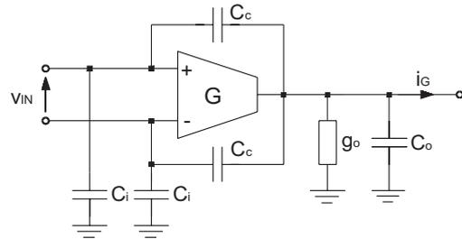
Fig. 7. Transconductor model including parasitic conductance and capacitors
