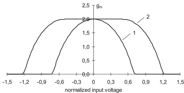
Fig. 6. Theoretical transconductance characteristics for (1) simple differential pair transconductor, (2) linearized transconductor
