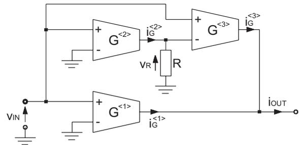
Fig. 3. Three-block feedforward transconductance amplifier
