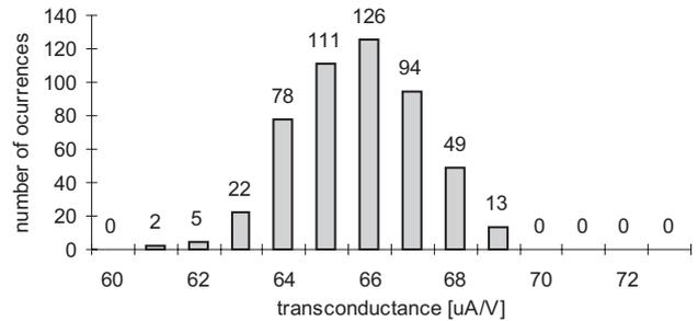
Fig. 13. Monte-Carlo simulation results for transconductance of OTA in Fig. 9 for  $I_{bias} = 40\mu\text{A}$  and 1% deviations (with gaussian distribution) in  $V_{th}$  and  $k$
