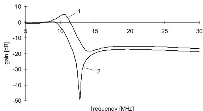
Fig. 17. Amplitude characteristic of 3<sup>rd</sup> order elliptic filter in Fig. 16: (1) without phase compensation, (2) with phase compensation of OTA
