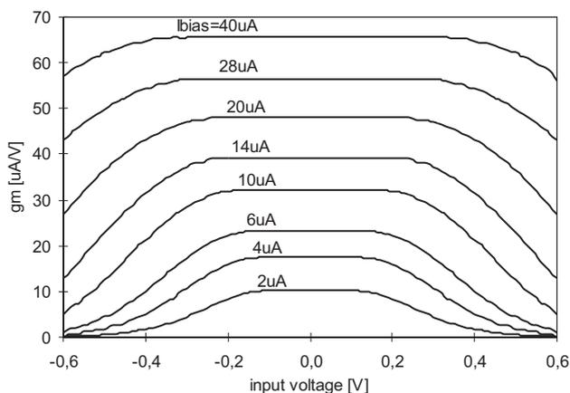
Fig. 14. Transconductance tuning capability for OTA in Fig. 9
