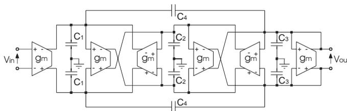
Fig. 16. Diagram of the 3<sup>th</sup> order low-pass elliptic  $G_m$ -C filter in LF structure with floating capacitor
