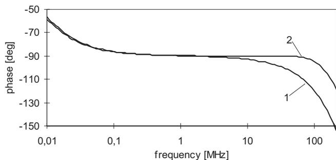
Fig. 15. Phase characteristic of OTA-C integrator with 1pF load (1) without phase compensation, (2) with 0.035pF compensation capacitor
