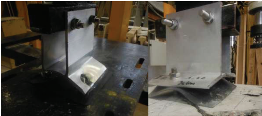
Fig. 5. Damaged aluminium brackets after tensile tests
