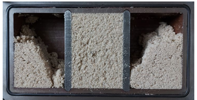
Fig. 5. Visualization of filling the core box sectors for a shooting pressure of 0.3 MPa and a blow hole diameter of 25 mm with the classic method of shooting [15]
