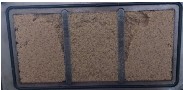
Fig. 7. Visualization of filling the core box sectors for a shooting pressure of 0.5 MPa and a blow hole diameter of 25 mm, for an integrated process (with pressure p = -0.1 MPa, relative to atmospheric pressure) [15]
