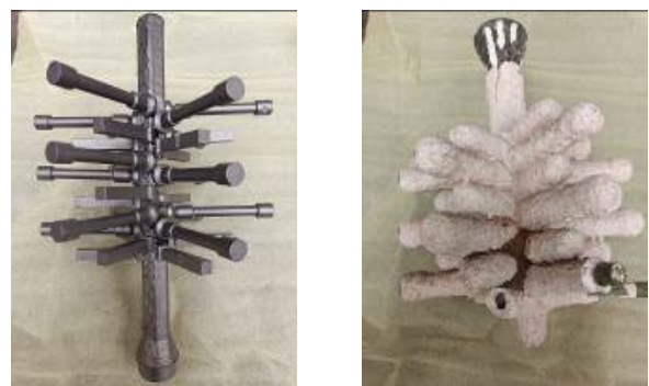
Fig. 3. Low pressure die-cast tree (a) and gravity cast tree with shell (b)
