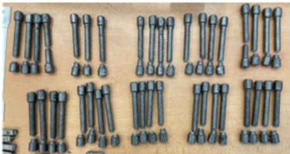
Fig. 5: Tensile test samples after test implementation
