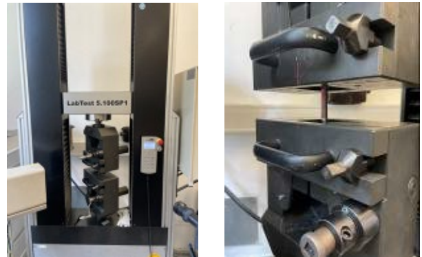
Fig. 2. Tensile test on the machine LabTest 5.100SP1 (a) and a view of the specimen mounted in the machine chuck (b)
