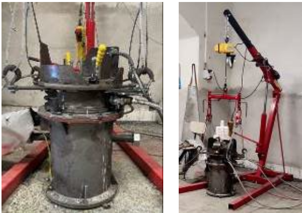
Fig. 1 Experimental NTL device (a) and assembly of the ceramic mould on the device (b)
