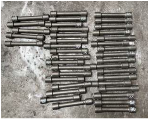
Fig. 4: Separated samples from trees for tensile test
