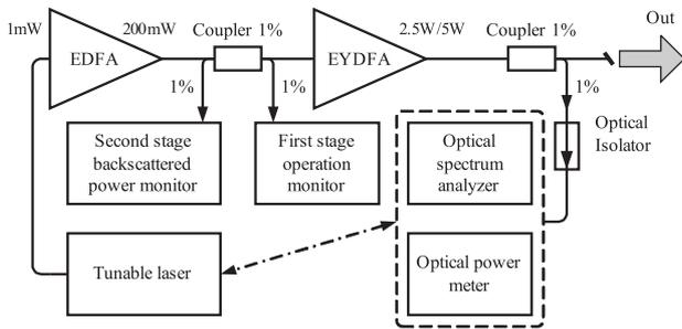
Fig. 5. Measurement circuit for the built MOPA configuration
