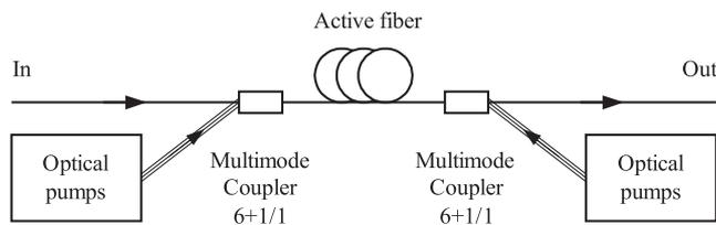
Fig. 3. Second stage of the amplifier cascade
