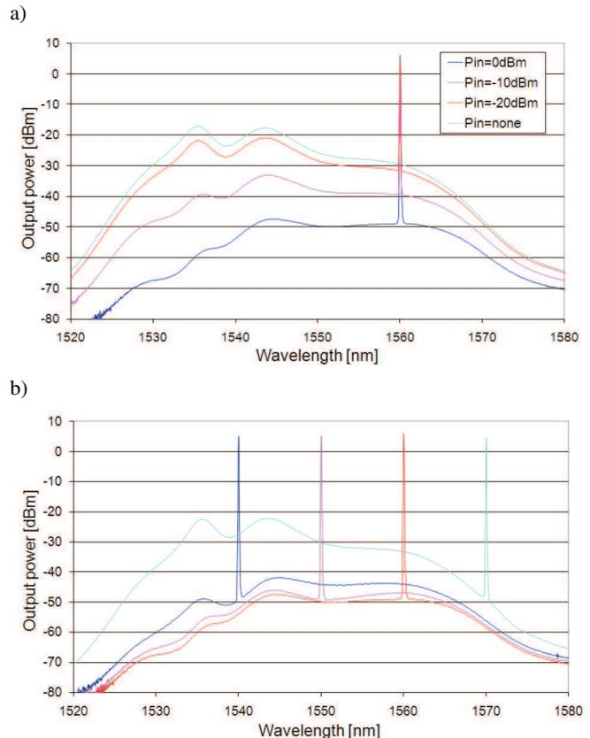
Fig. 7. Optical spectrum of output signals: a) ASE noise on the cascade output vs. input signal power, b) output signal spectrum for four wavelengths for 0 dBm input power
