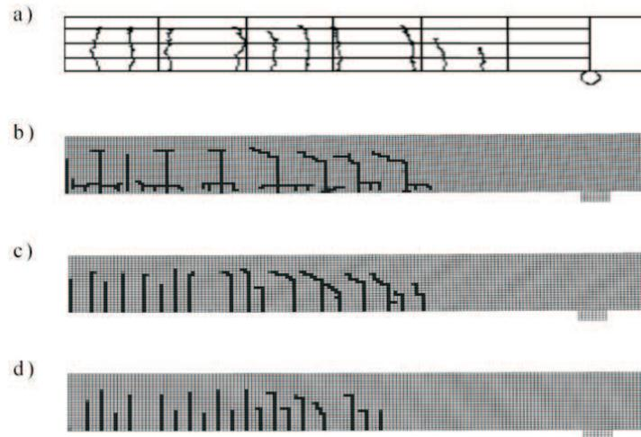
Fig. 8. Distribution of beam damage (at 24 kN load): a) experimental result, b), c), d) numerical results.
