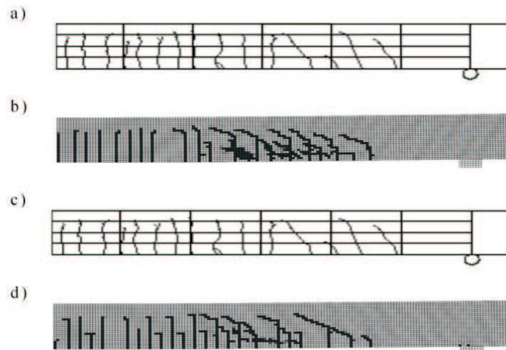
Fig. 9. Distribution of beam damage (at 47 kN load): a), c) experimental results, b), d) numerical results.
