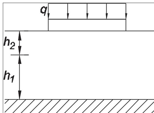
Fig. 7. Thick plate on two-layered foundation.
