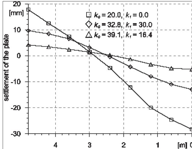
Fig. 3. The settlement of the plate along  $x$ -axis for uniformly distributed load.
