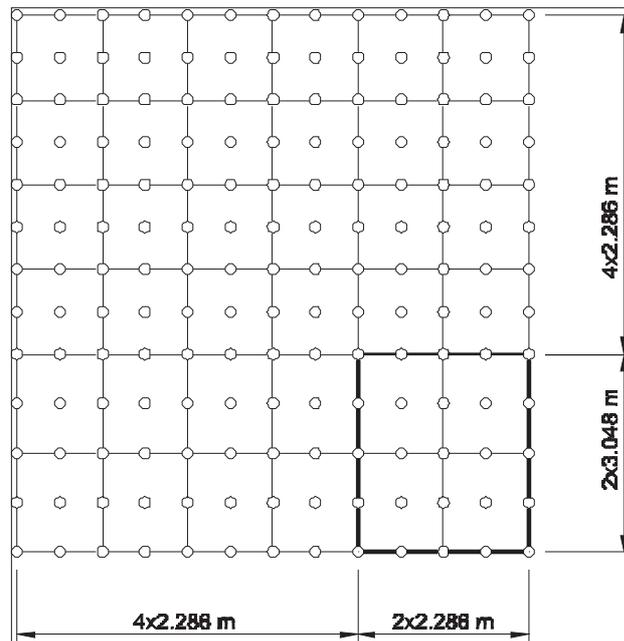
Fig. 4. Free rectangular plate on elastic foundation (only one quadrant is discretized).
