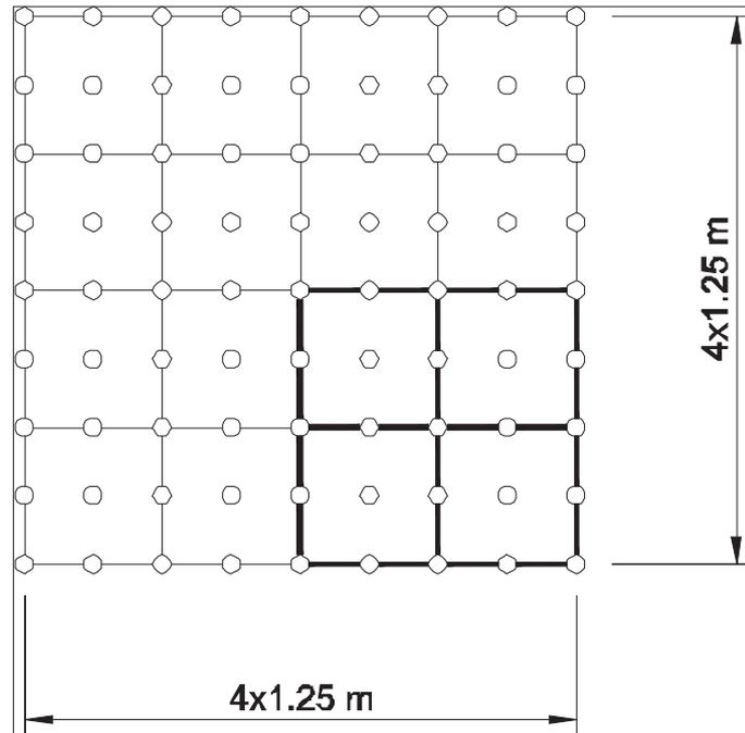
Fig. 6. Arrangement of square plate on elastic foundation.
