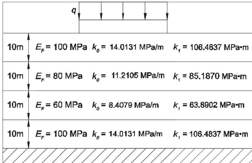
Fig. 9. Thick plate on four-layered foundation.
