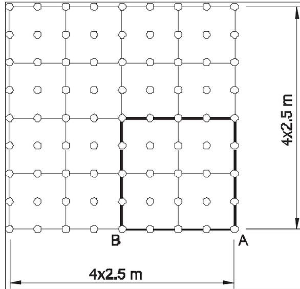
Fig. 8. Finite element discretization of square plate.
