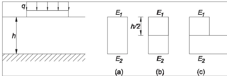
Fig. 5. Free plate: (a) one layer,  $E_2 = E_1$ , (b) two layers,  $E_2 = E_1$ , (c) two layers,  $E_2 = 2E_1$ .
